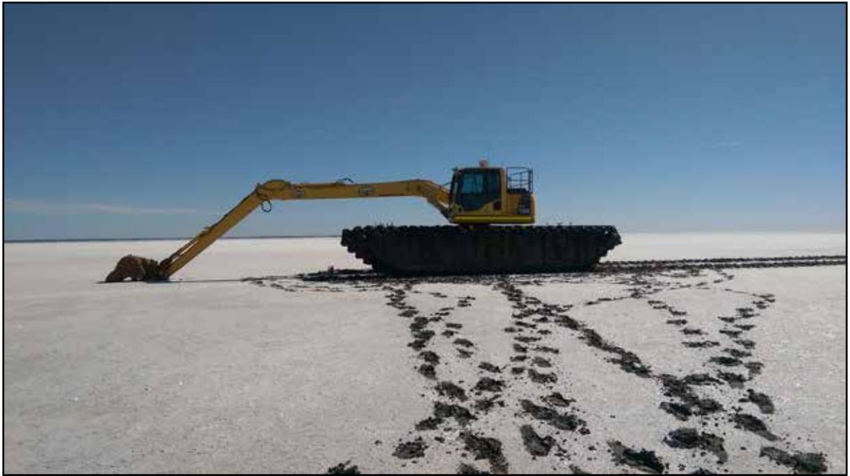
These excavators are able to float on the surface of a lake or work in extremely boggy conditions, where a normal machine could not.
